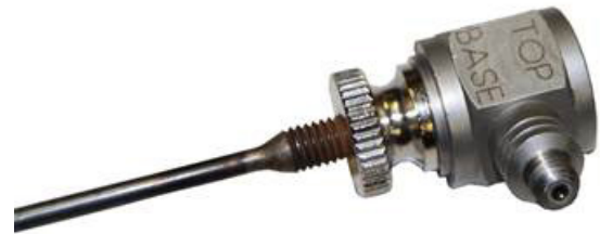
Figure 2: Force transducer (shown installed on a modal stinger)
